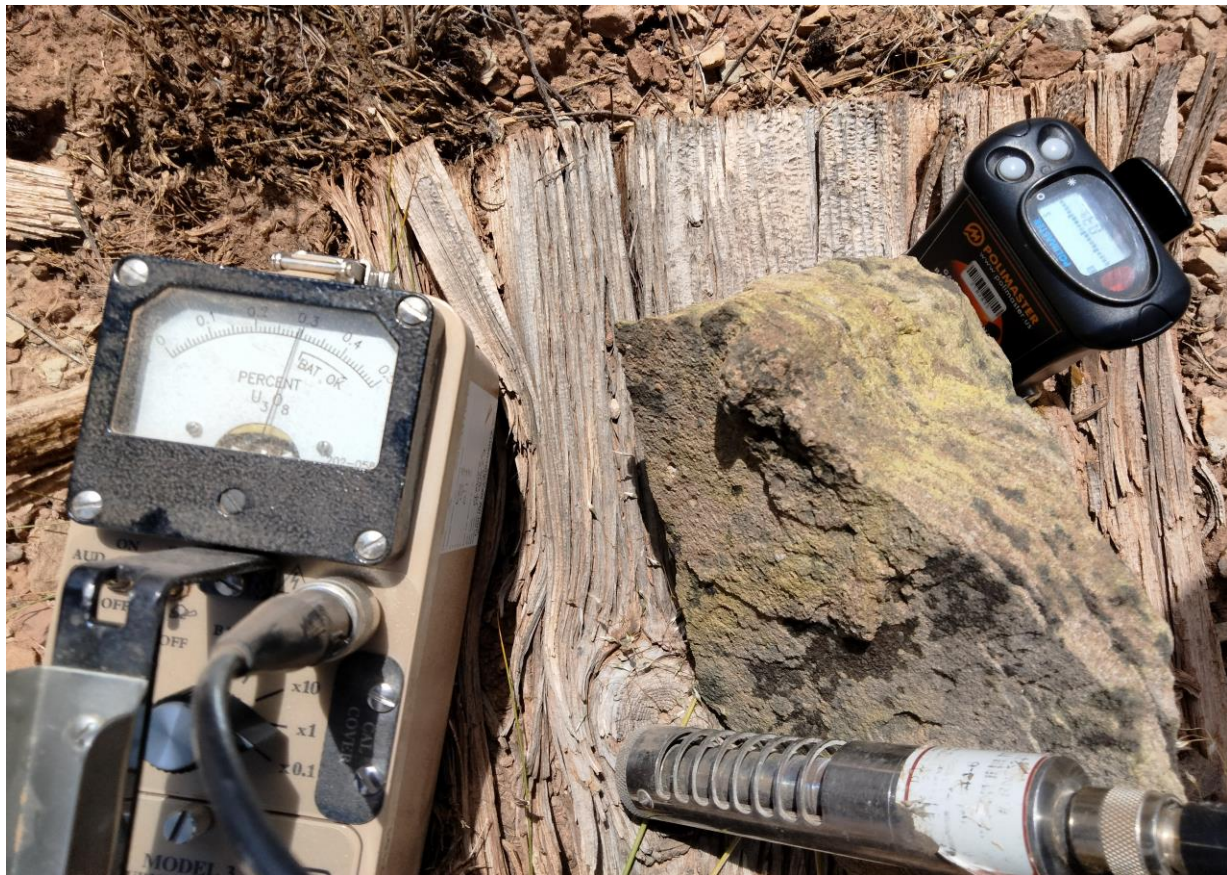
Photo 12.1: Sample 650470 from an unnamed dump on the Fawn claim block. Highly visible carnotite grades 0.3% U 3 O 8 in the Ludlum Model 3 Geiger counter. The laboratory assay returned 4867 ppm U (0.49% U 3 O 8 ) and 3120 ppm V (0.557% V 2 O 5 ). Important associated pathfinder metals included 0.5% Ba and 9.4 ppm Mo.
