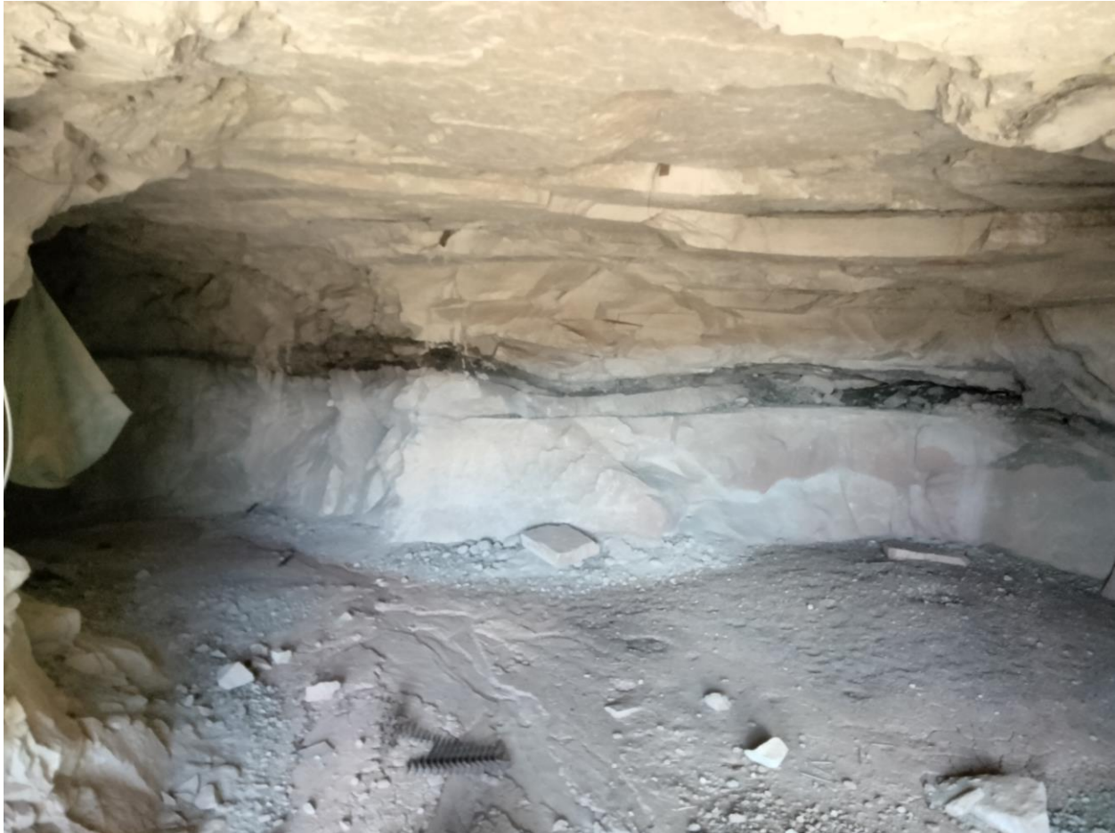
Photo 6.1: An unnamed portal on the Slick S claim block showing the U-V mineralized zone in the working face. Sample 650467 from the adjoining dump assayed 1020 ppm U (0.118% U_3O_8 ) and 1080 ppm V (0.179% V_2O_5 ).
