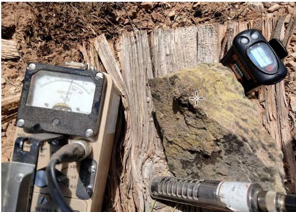
Photo 12.1: Sample 650470 from an unnamed dump on the Fawn claim block. Highly visible carnotite grade 0.3% U_3O_8 in the Ludlum Model 3 Geiger counter. The assay returned 4867 ppm U (0.49% U_3O_8 ) and 3120 ppm V_2O_5 (0.557% V_2O_5 ). Important associated pathfinder metals included 0.5% Ba and 9.4 ppm Mo.
